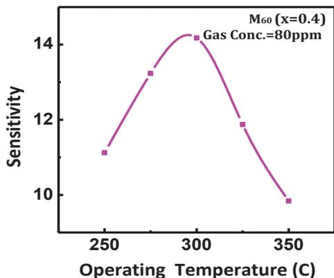
Fig. 3. Variation of sensitivity with operating temperature for typical sample
