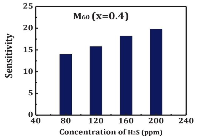
Fig. 6. Variation of sensitivity with concentration of H<sub>2</sub>S Gas for typical sample
