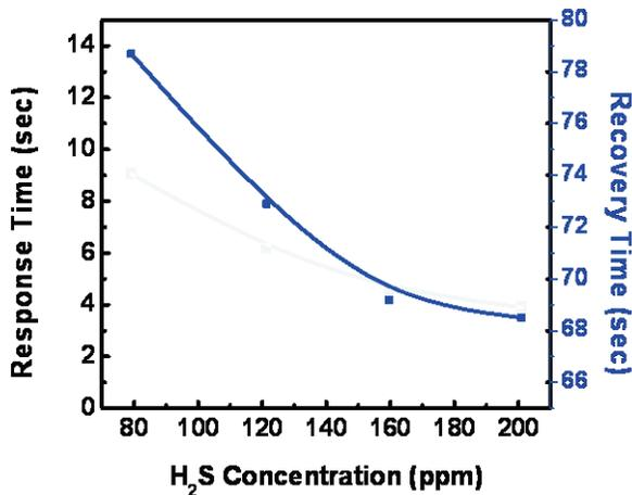
Fig. 5 Variation of response and recovery time with gas concentration
